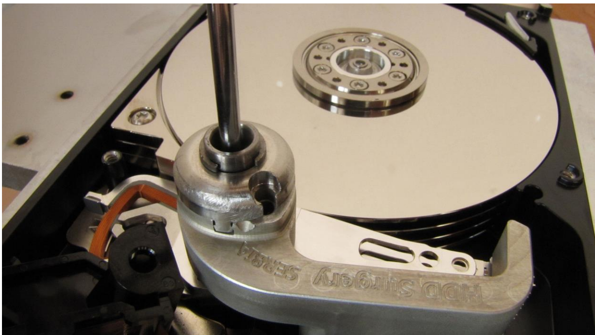
Picture 6. (unscrewing the head assembly)
