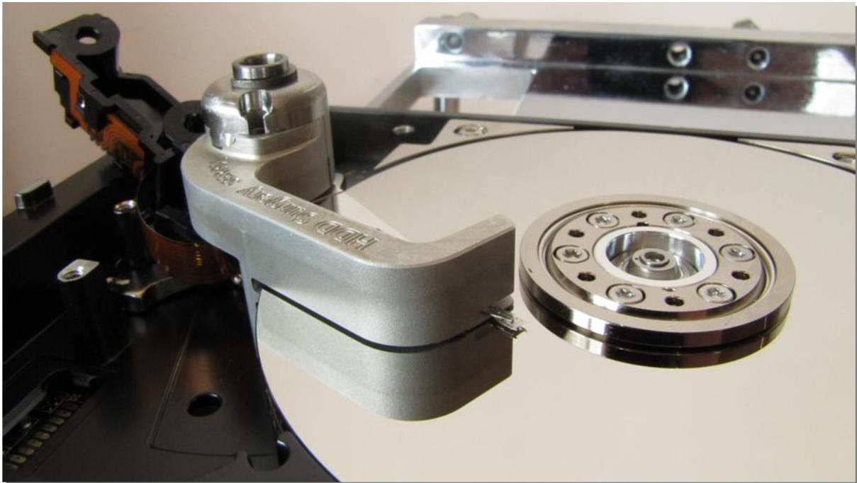
Picture 9. (moving the heads to their place)
