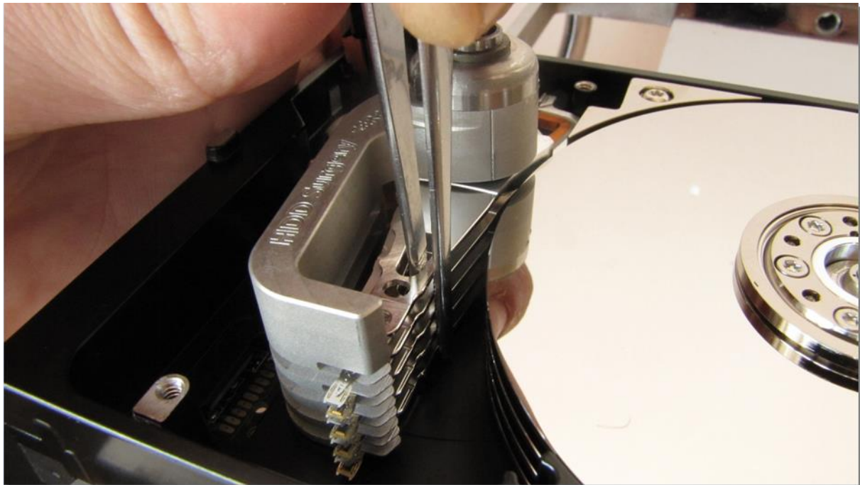
Picture 8. (mounting the heads on a patient drive)
