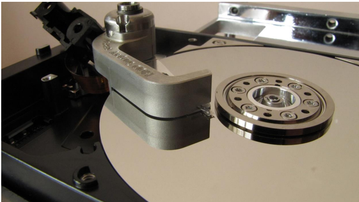
Picture 3. (lifting the heads)
