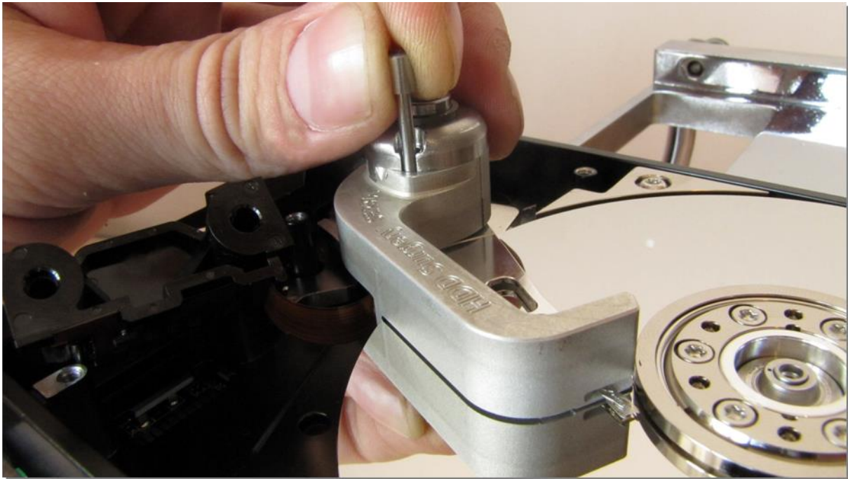
Picture 10. (remove the securing pin)
