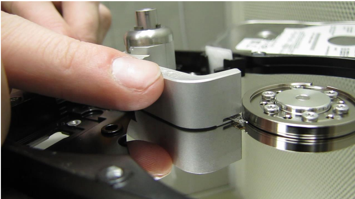
Picture 3. (lifting the heads)
