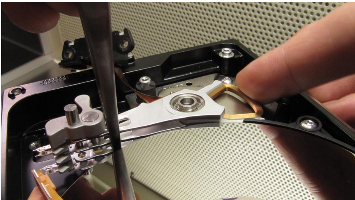
Picture 10. (mounting the heads in a patient drive)
