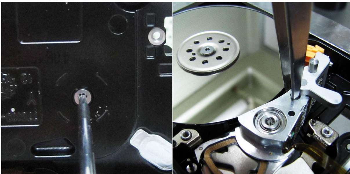
Picture 16. (dismounting the heads on 2.5" hard drives with 4 platters)
