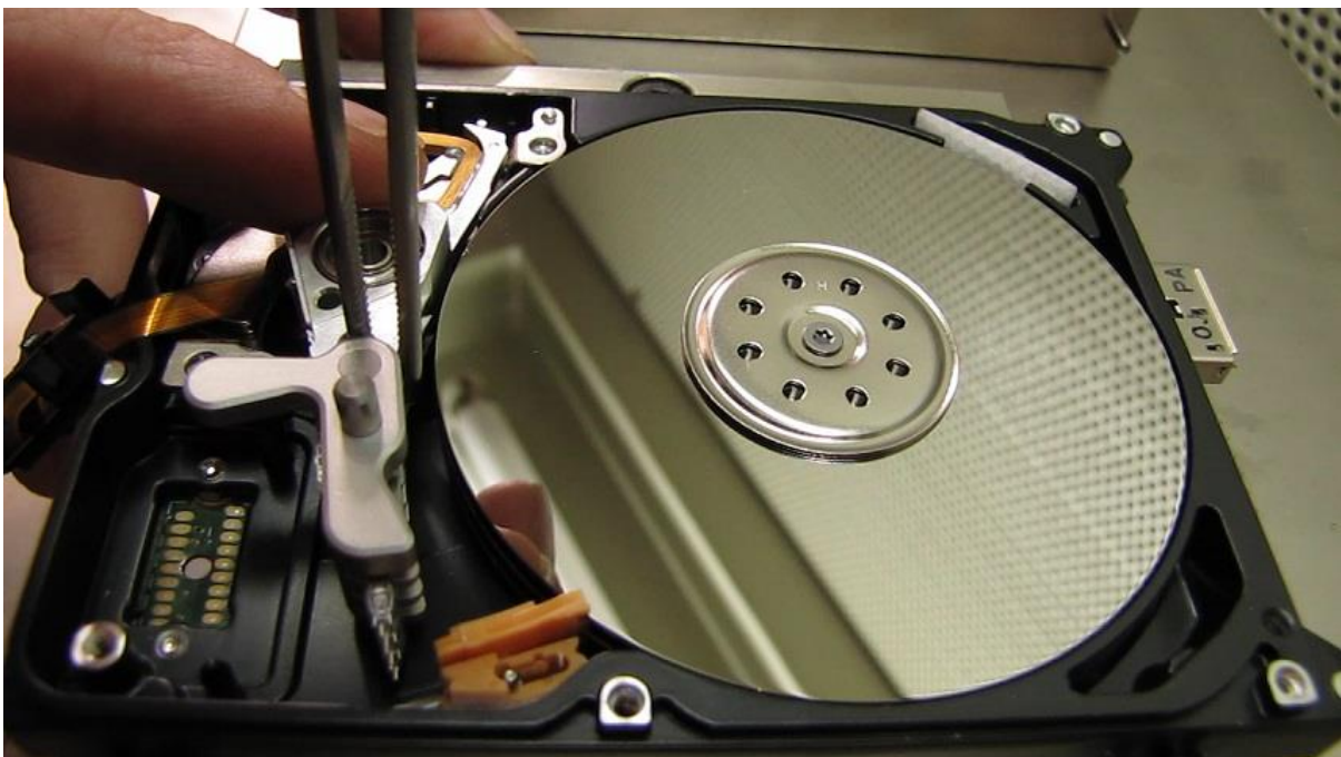
Picture 13. (mounting the heads in a patient drive)
