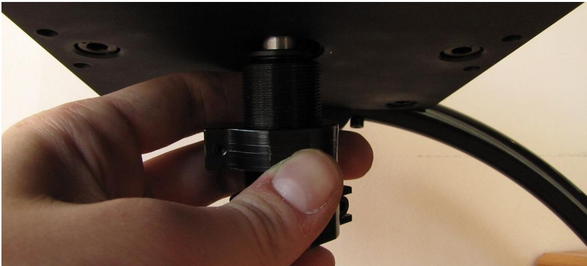
Screwing the bottom cylinder with cocoon and bearing
