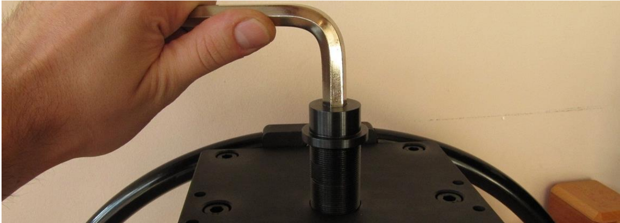
Pushing out the bearing from hard drive casing
