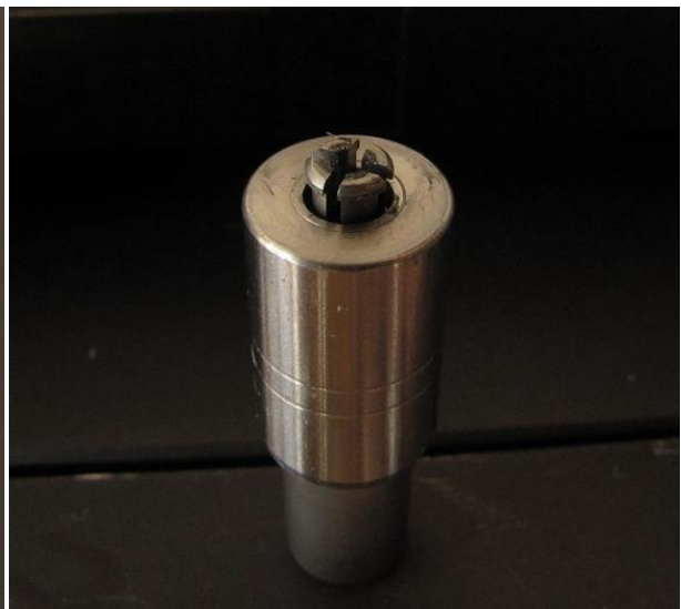
“The puller” with bearing casing
