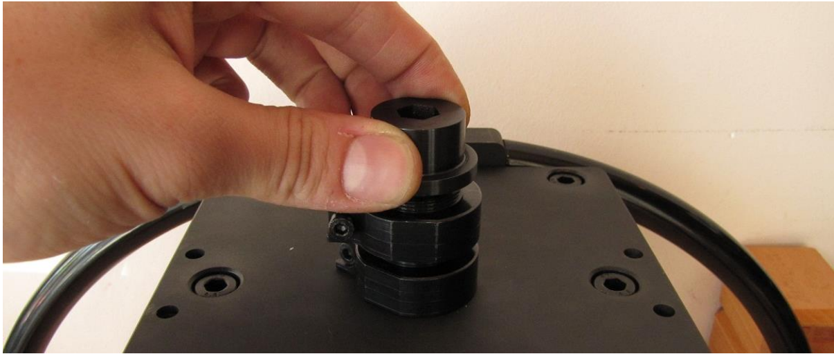
Screwing the spindle-pushing screw
