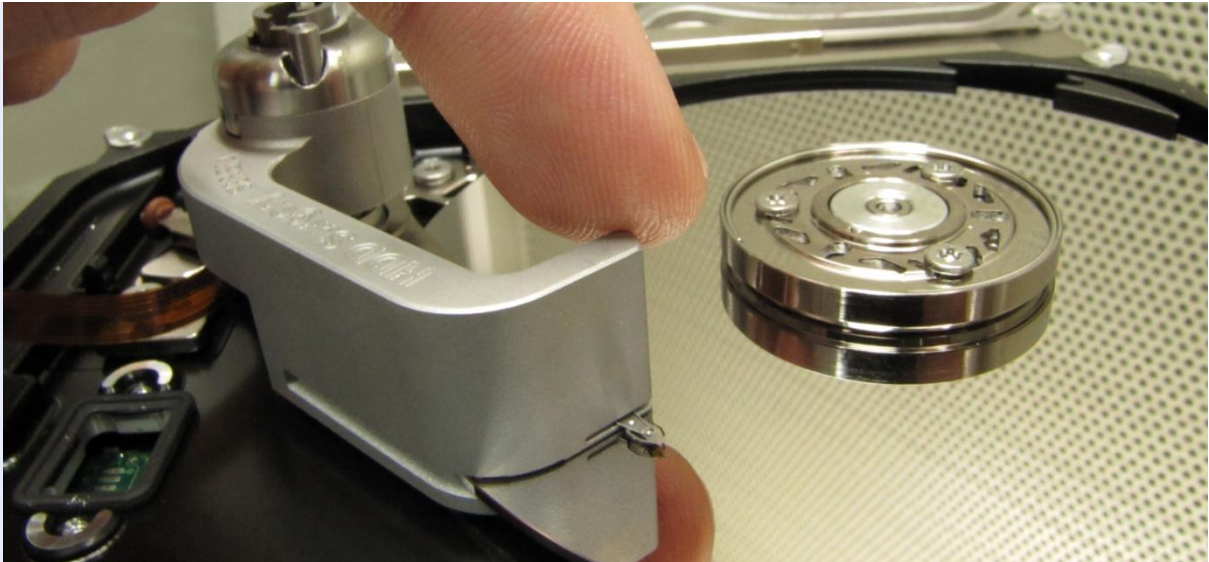
Picture 5a. (Moving secured tool with heads outside of platters area)
