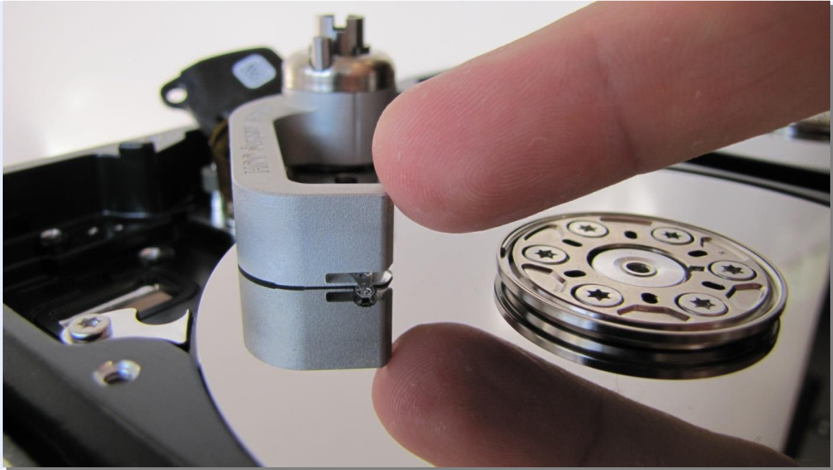
Picture 5. (moving secured tool with heads outside of platters area)
