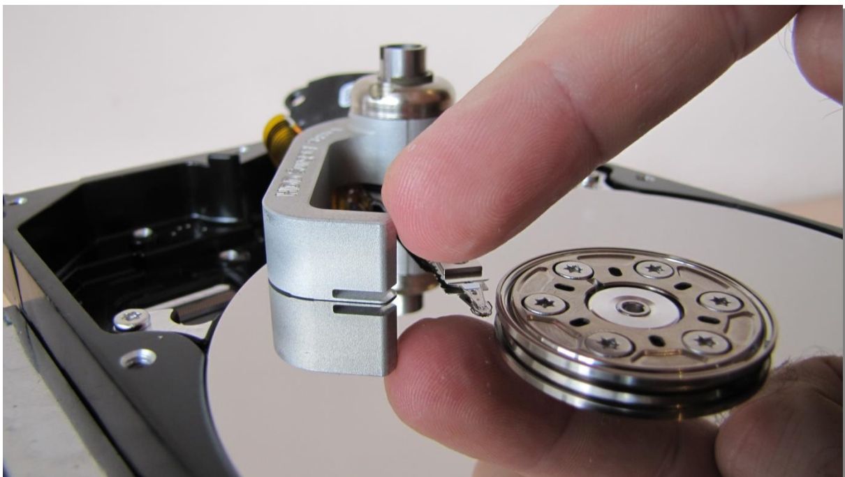
Picture 9. (returning the tool outside of platters)
