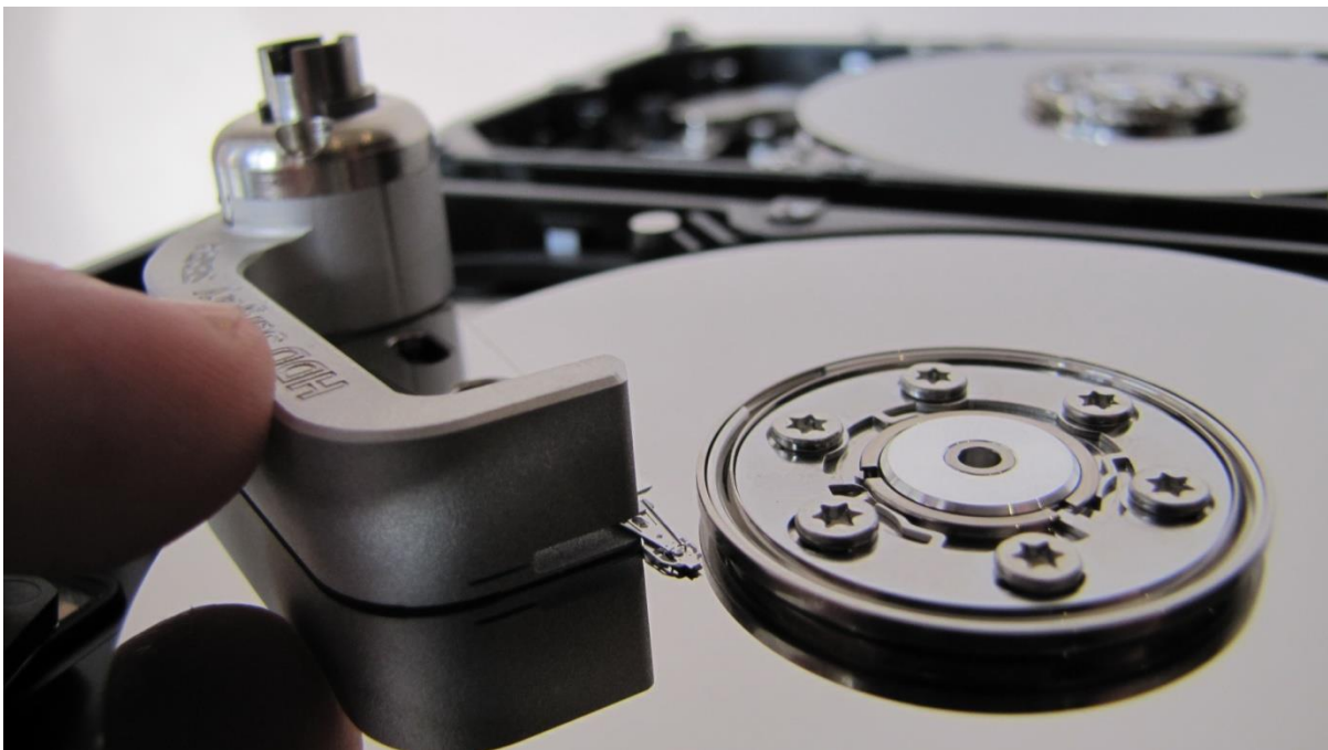
Picture 3. (lifting the heads)
