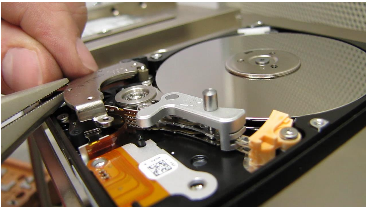
Picture 14. (moving the heads to the ramp)
