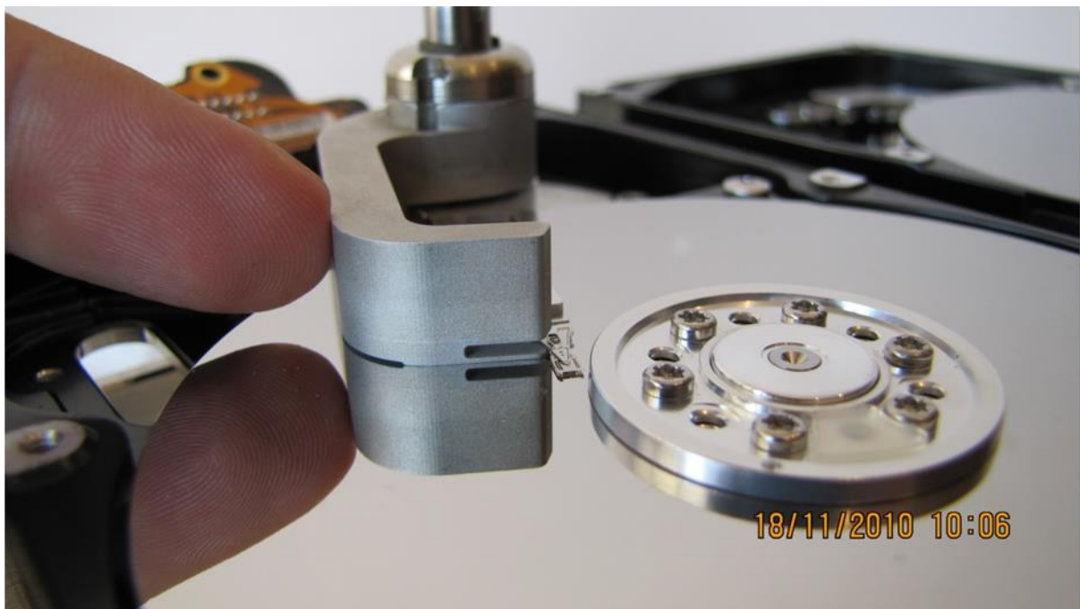
Picture 3. (lifting the heads)
