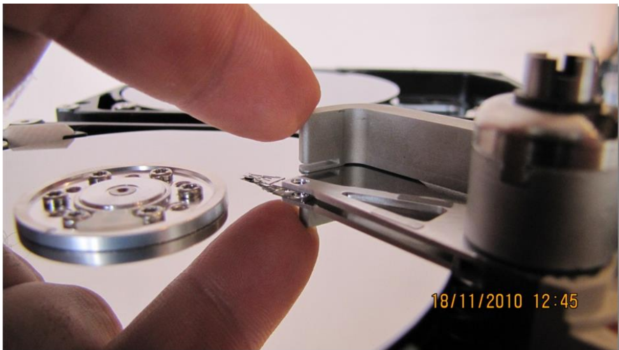
Picture 9. (returning the tool outside of platters)
