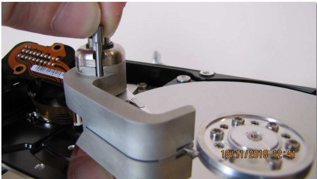
Picture 8. (remove the securing pin)
