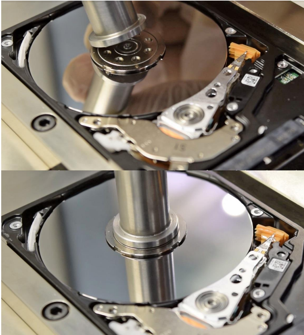
Picture 3.2. Positioning the base on the surface of the platter holder
