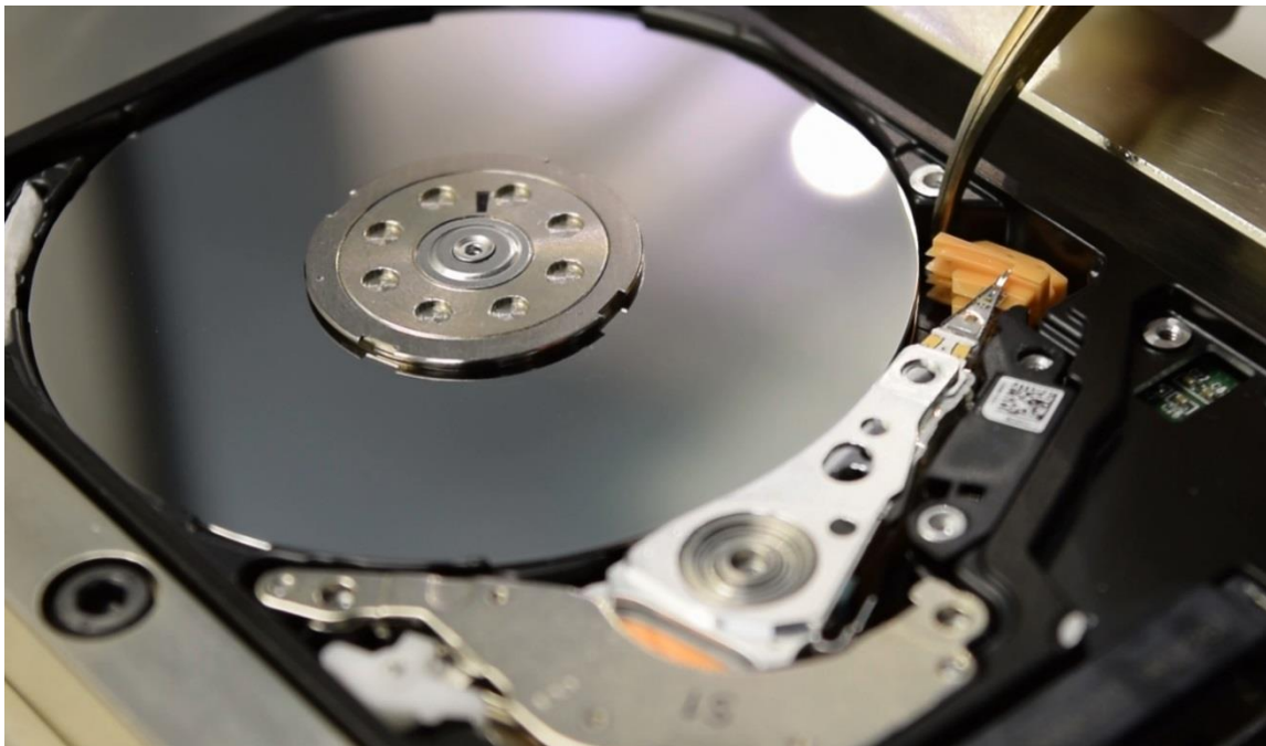
Picture 3.1. Removing the ramp
